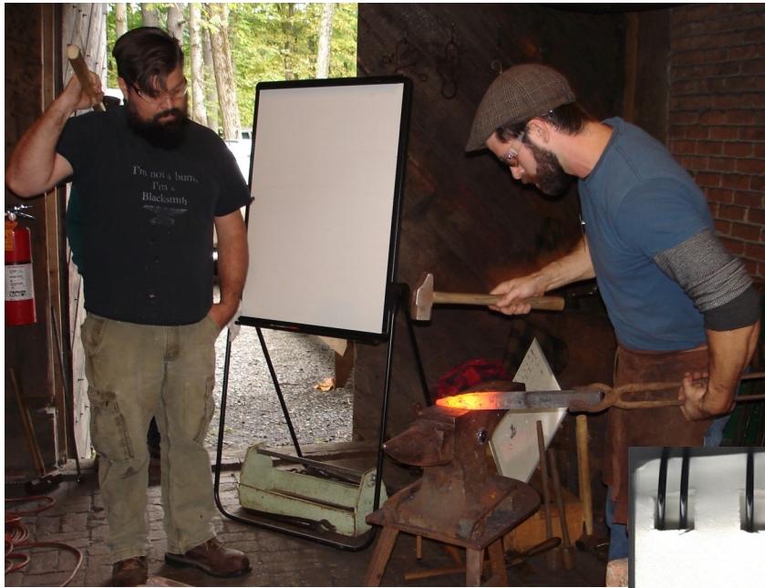
Tim Miller stands by ready to strike for Eric as he refines a taper.
